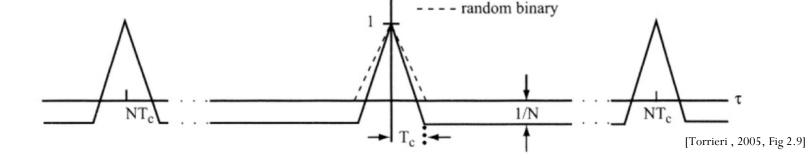
$\bullet\,$  Power spectral density of maximal sequence.
